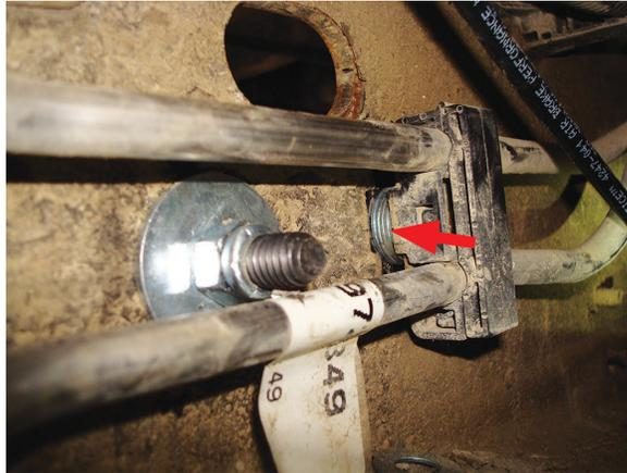
4 X 5/16" washers (P) stacked up behind line holder's in the front and in the rear of axle.
